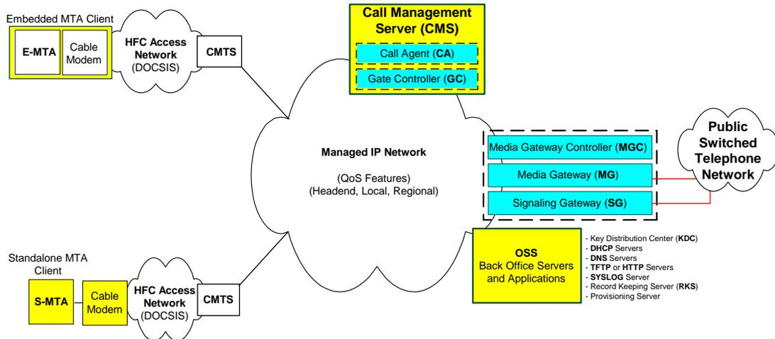
Figure 2. IPCablecom 1.0 Network Component Reference Model
