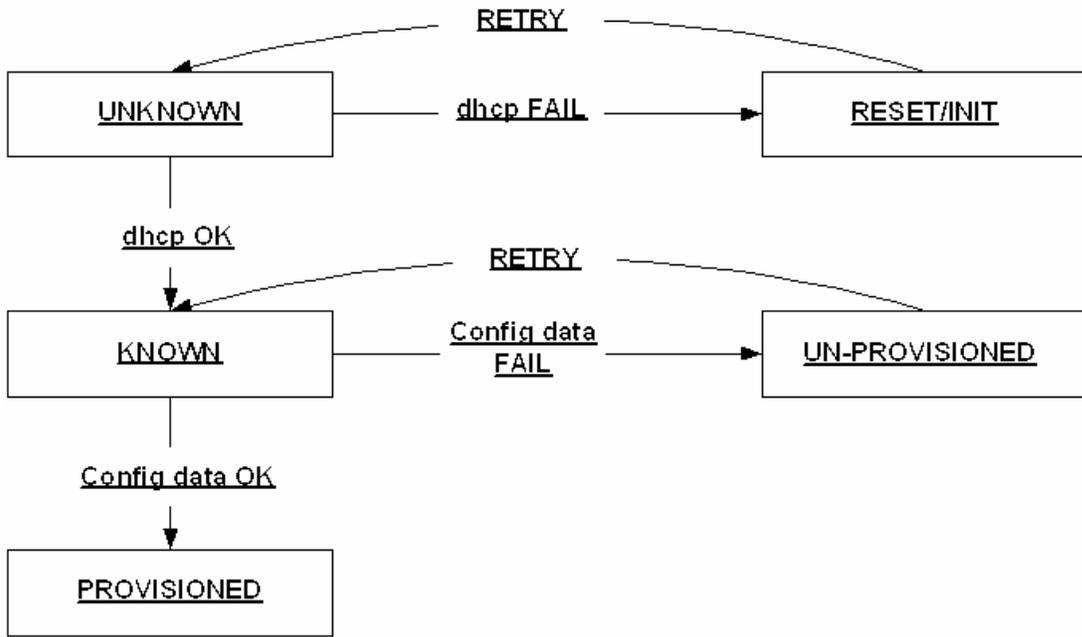
*Figure 5. Device States and State Transitions for Basic and Hybrid Flow Provisioning*
