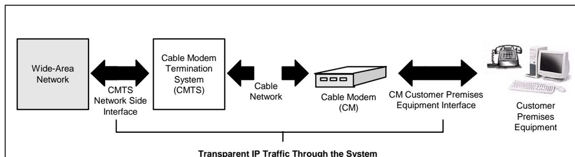
*Figure 1. Transparent IP Traffic Through the Data-Over-Cable System*
